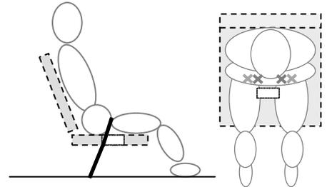
Containment Seats with Crotch belt mounting directly to seat bottom OR through holes provided at the back of the seat bottom: (*Driver is sitting on the Crotch belts*)
